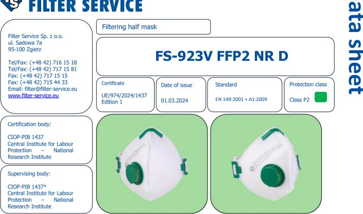
For protecting the user's respiratory tract against the harmful impact of air pollution in the form of solid and/or liquid particles forming aerosol (dust, fumes, mists) up to  $10 \times TLV$ .
